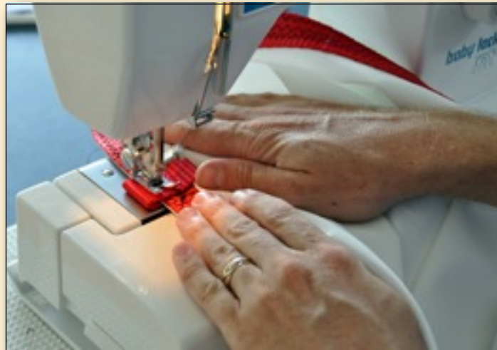
Much of the sewing was done using a heavy duty BabyLock machine which handled Odyssey III with no problems. Over two layers of polyester, webbing bolt-rope presented a challenge, and eventually forced Barry to borrow a sailmaker's walking foot machine.
