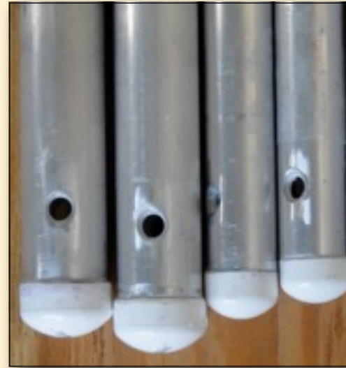
The ends of some of the mizzen battens, with PVC ends and caps epoxied in to keep the water out and protect whatever they are bouncing onto.
